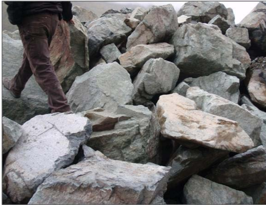
Figure C - 5. Stockpile of Large Stone Consisting of Two-Foot to Five-Foot Diameter Boulders
